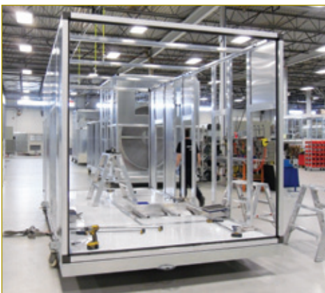
A unit with aluminum interior lining under construction on the assembly line.
