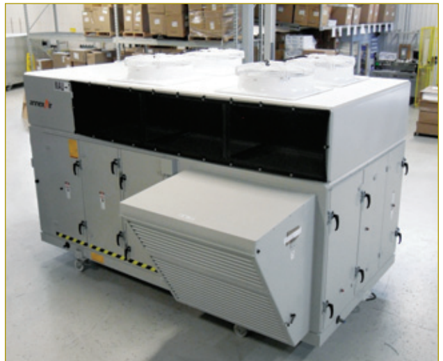
This 100% Outside Air MAU 46 ton unit can modulate from 7 to 46 tons. All integrated ACCU units include a protective nylon mesh in front of the condenser coil; this protective screen is auto-cleaning to ensure maximum coil performance.
