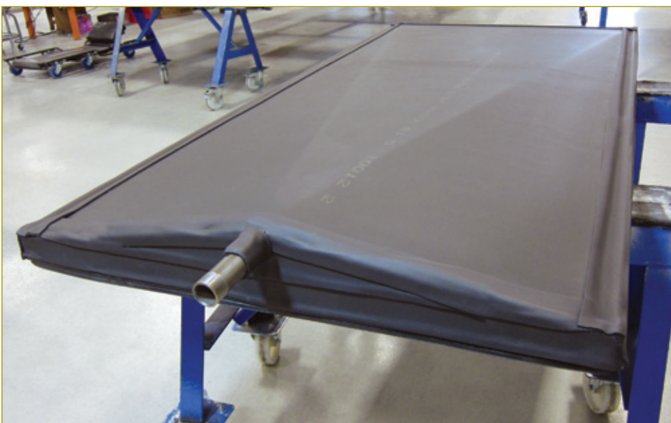
All condensate drains are carefully insulated with a self-adhesive 0.5 in. EPDM membrane also placed on the sides and a portion of the drain.
