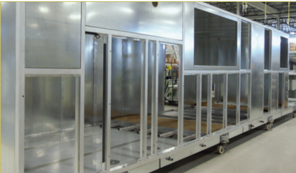
Example of a 30,000 CFM AHU unit with 160 ton ACCU.
