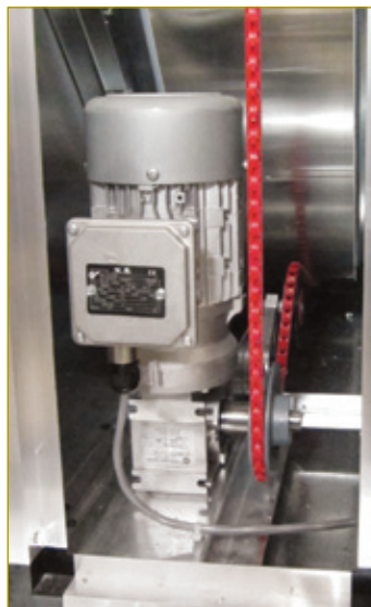
The reinforced fiberglass wheel belt is a Power Twist type from Fenner Drive. This belt is indestructible!
