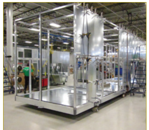
A standard unit construction incorporating aluminum profiles and double wall G90 galvanized steel panels.
