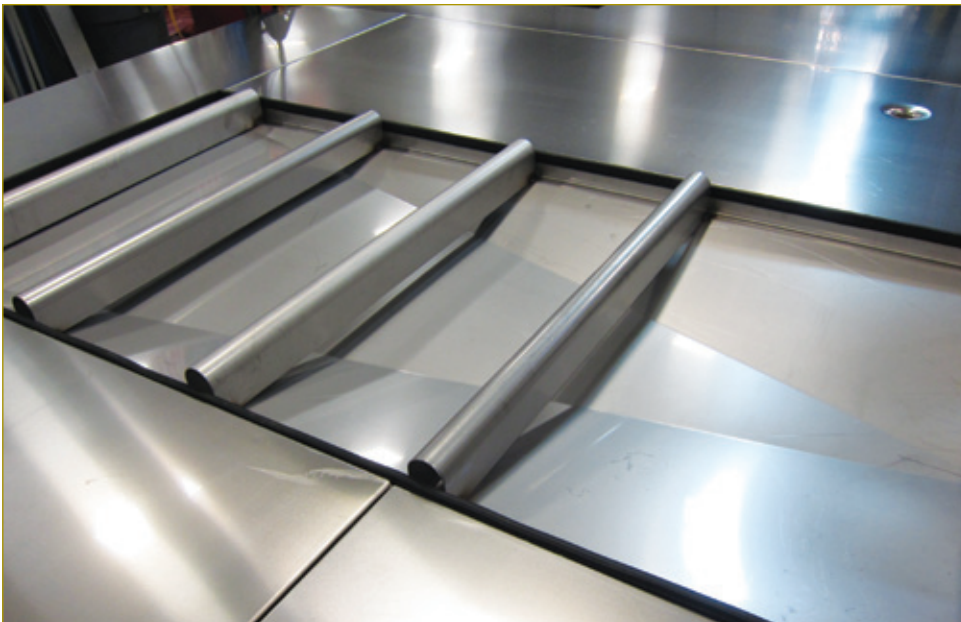
All condensate drain pans are built with a 3 sided incline slopes and are made of heavy gauge 304 stainless steel.
