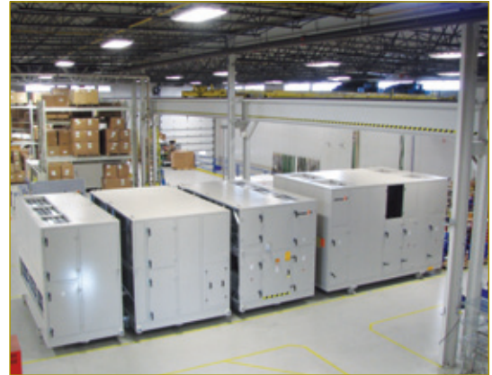
Annexair's design flexibility allows us to build units as a single piece or with multiple modules. Example of a 25,000 CFM modular unit with heat wheel during the wiring process.
